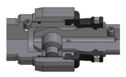
Cardan Joint: Cardan joint is the best solution for heavy application with high pressure inside the pump casing. It improves the allowable torque up to 4 times torque with the same pump size. It is available with internal metal joint protection to for an additional improvement of the rubber service life.
