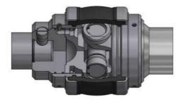
Joint protection: In the DHB e JHB series the joint rubber sleeve and clamp are protected from a particular device integrated inside the end of the auger feed screw. This characteristic is of considerable importance because it ensures the integrity of the joint in the case of pumping of abrasive substances or with solid blunt, without the needed to add expensive optional components.
