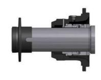
The type of seals is interchangeable on the standard pump. Each solution was carefully engineered while taking into consideration all the operating conditions. As well as changing the sealing system, you can also install various types of mechanical seals based on the application.
