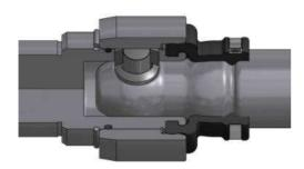
Cardan Joint: Cardan joint is the best solution for heavy application with high rotation speed and high pressure inside the pump casing. It improves the allowable torque up to 4 times torque with the same pump size. It is available with internal metal joint protection to for an additional improvement of the rubber service life.
