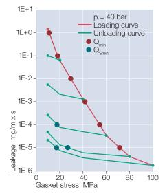
Q<sub>A</sub> = Stress on the gasket during installation before unloading
