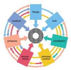
A statement about the expected tightness of the flange connection is only possible if a qualified and defined installation of the gasket has been executed.
