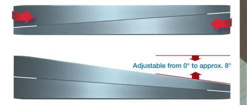
Slant positions occur with all flange connections.
