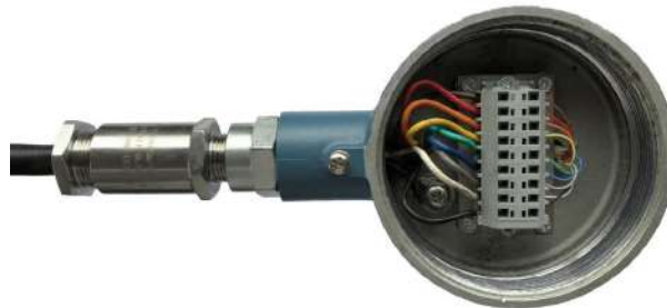
Fig.4.9 Nine-core shielded cable connection
