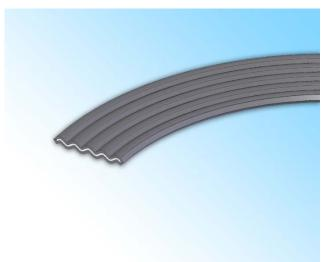
Klinger Maxigraph consists of a corrugated metallic core encapsulated by a graphite coating. Excellent microsealing performance from the graphite is combined with the strength of the metallic core.
