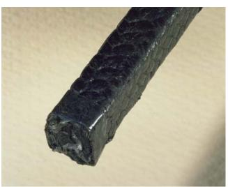
A combination of selected glass fibre yarns with graphite lubricant impregnation, Klingerlock braided to produce an efficient alternative to asbestos in valve applications and static sealing duties eg. caulking purposes.
