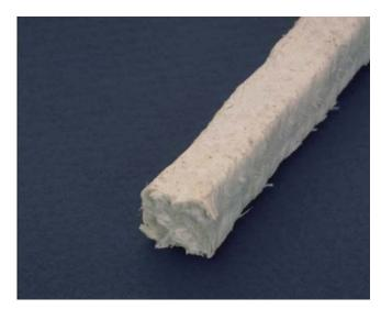
A combination of selected glass fibre yarns with PTFE impregnation, Klingerlock braided to produce an efficient alternative to asbestos in valve applications and static sealing duties e.g. caulking purposes.
