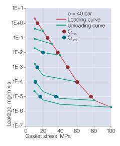
$Q_A = Stress$  on the gasket during installation before unloading
